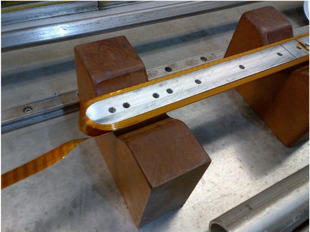
Figure 6: A photo of the 20 turn pole winding after fabrication on the winding machine. The 12 mm wide HTS tape conductor with its Kapton CI wrap is visible on the left. The next step in the construction process was to heat the winding in a controlled oven to 225 °C in order to activate the polyimide adhesive of the Kapton CI. Before testing in liquid nitrogen, current leads and voltage taps were attached to this winding, then it was mounted back on its mandrel and secured with various restraints.
