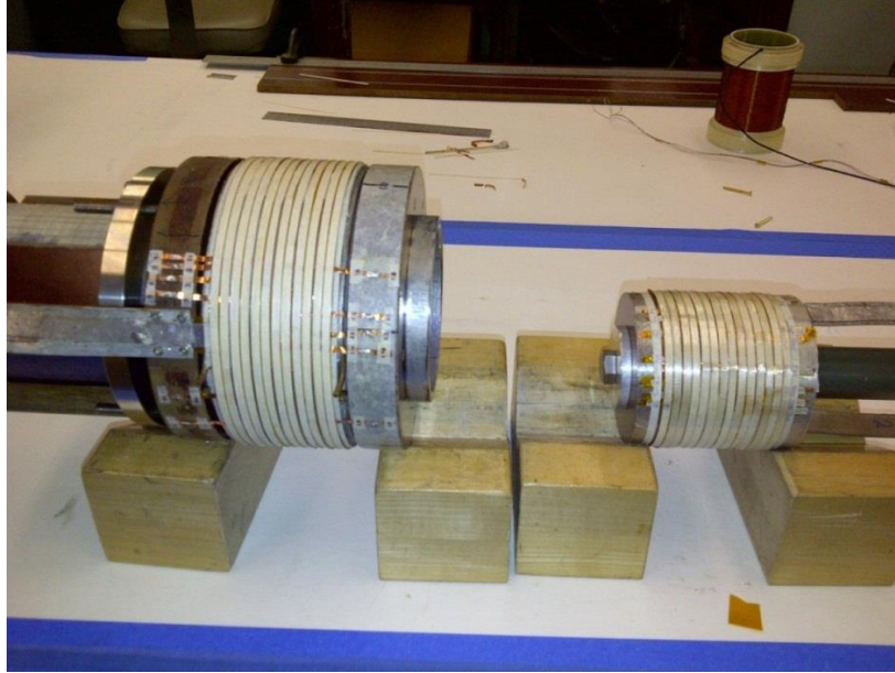
Fig. 5a. Left side—half-length “midsert” solenoid of 12 YBCO pancakes that generated a maximum ambient field of \sim 9.2 T at 4 K. Right side—14-pancake YBCO “insert” magnet that generated nearly 16 T on axis. Neither magnet quenched.
