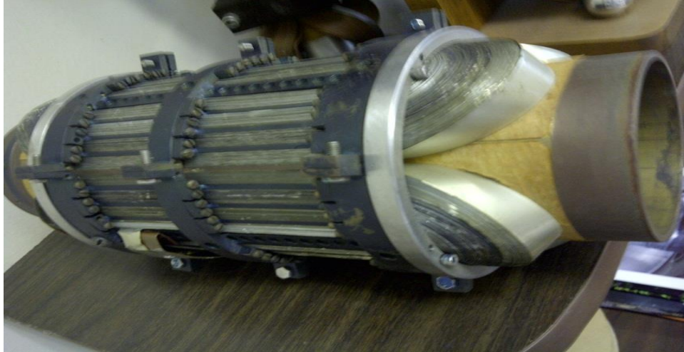
Fig. 4. Nb 3 Sn tape quadrupole made by W. Sampson at BNL.
