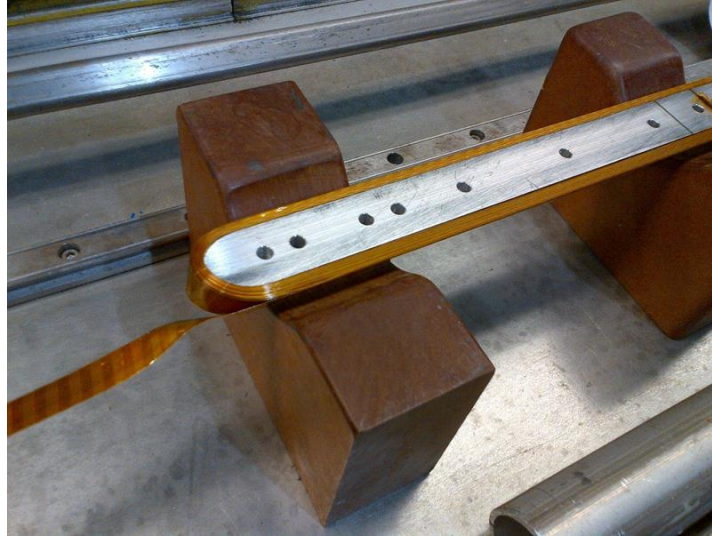
Fig. 3. The coil winding made in the previous Phase 1. An actual magnet would be made of a series of such windings filling the circumference of the tooling mandrel, separated by wedges to control field shape.
