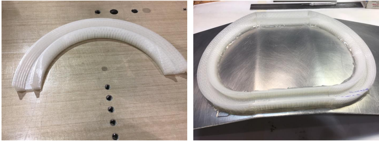
Figs. 10a&b: Spacers made by a 3-D printer. Left: A quasi-semicircular arc. Right: Complete assembly.
