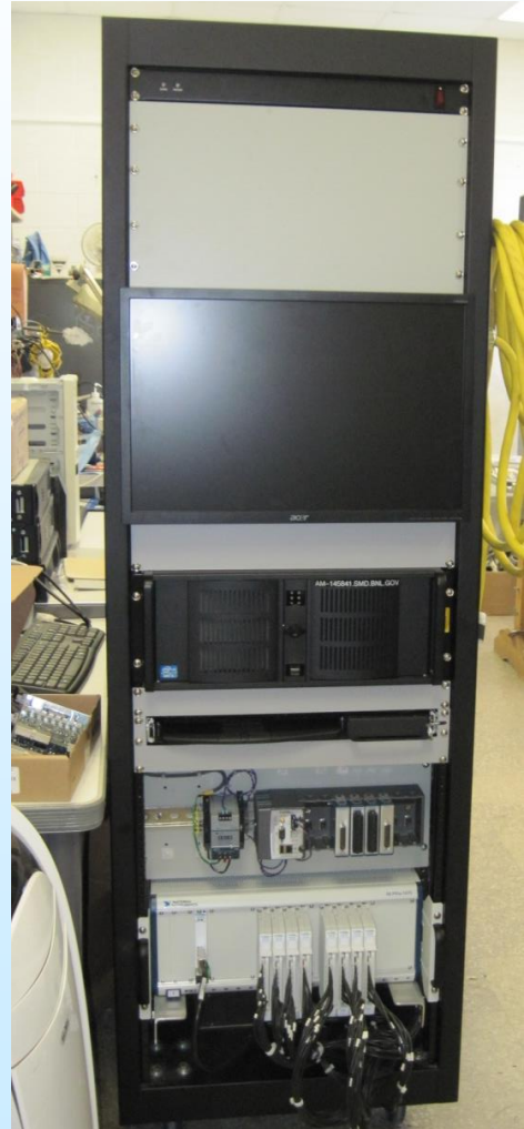
Cabinet #2 (32 channels, 1kV) (expandable to 64 and 3kV)
