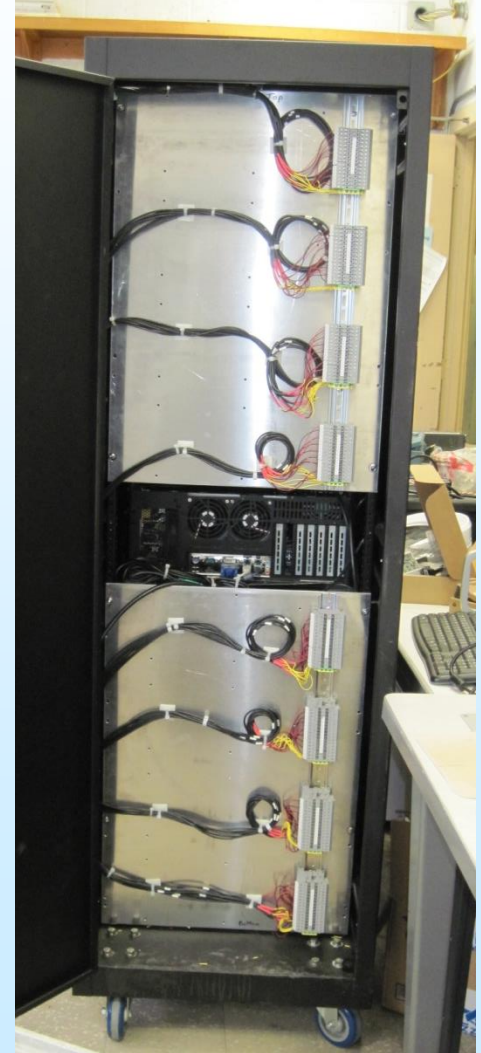
Cabinet #2 (32 channels, 1kV) (expandable to 64 and 3kV)
