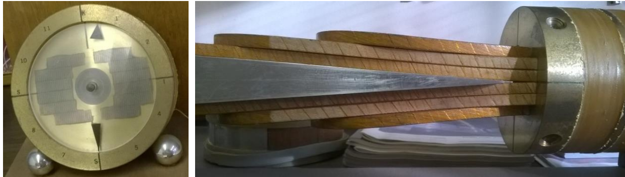
Figure 1.1: Nb 3 Sn block coil dipole with cross-section (left) and lifted ends (right).
