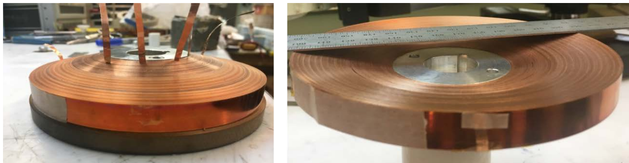
Fig. 8. Two views of the conical coil wound in Phase I.
