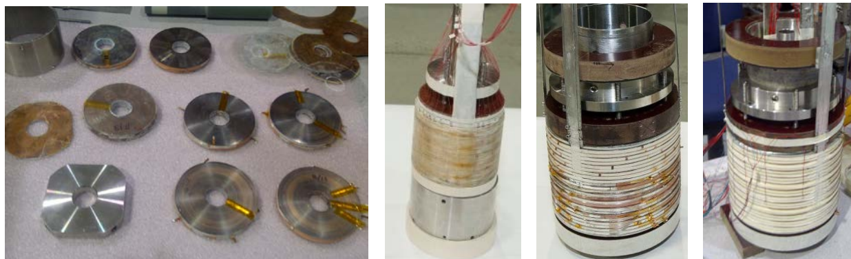
Fig. 1a-d.: High field HTS solenoids built and tested by PBL/BNL collaborations. Left: 25-mm bore pancake coils for insert magnet. Left-center: 7-double-pancake solenoid that generated 16 T. Right-center: Solenoid with 12 double pancakes of 100 mm bore. Right: Nested set. These coils are still available and use of them makes the demonstration of the novel 17 T solenoid design for neutron scattering possible in Phase II.
