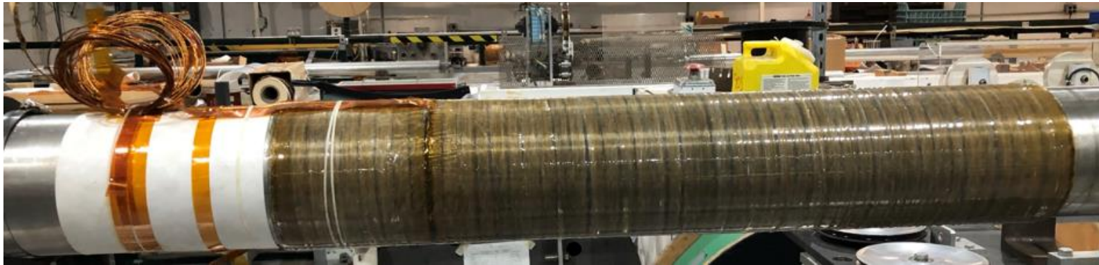
Double-layer tension wrapped and cured
